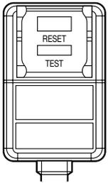
**TEST:** WHEN CURRENT LEAKING OR PRESSING TEST BUTTON, THE INDICATOR LIGHT WILL TURN OFF AND THE UNIT WILL CUT OUT.
